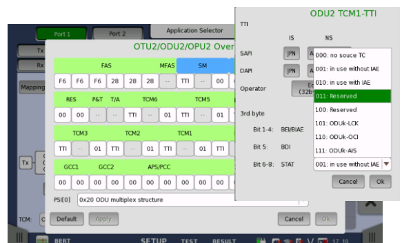
Figure 4. OTU transmitter Overhead
